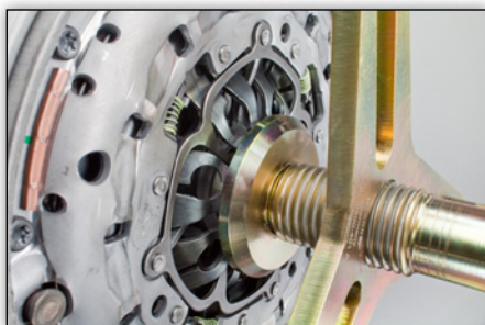
Image 8: Release the diaphragm spring by loosening the SAC tool spindle and remove the tool using the studs
