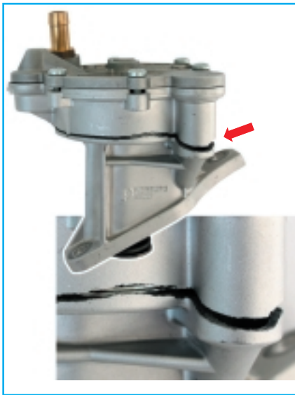
Fig. 1 Broken pump casing
